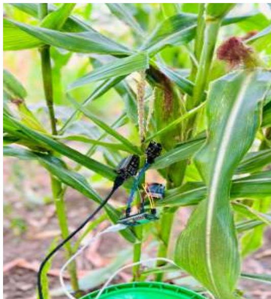
Figure 1 ultrasound sensors close to the plants to monitor their movements and inserted NPK sensors into the soil to monitor changes in the chemical makeup (Archana et al 2018)
